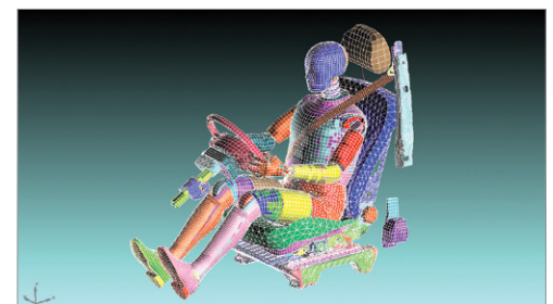
Dummy positioning and seat belt routing
